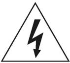
This symbol, wherever appears, is intended to alert the user to the presence of un-insulated dangerous voltage within the appliance's enclosure that may be of sufficient magnitude to a risk of electric shock.
